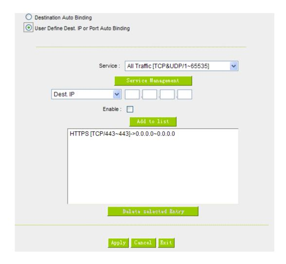
When any intranet IP connects with TCP443 port or any destination (0.0.0.0 to 0 represents any destination), it will go through the same WAN IP. As for which WAN will be selected, this follows the first- chosen WAN IP distributed by the original session balance mechanism. For example, there are two intranet IP-
